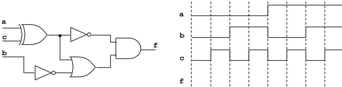
d) Complete the truth table describing the output of the following circuit and write the simplified Boolean equation (6 pts).
